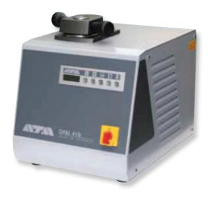
The Opal 410 is a fully hydraulic, water cooled hot mounting press for mounting samples before polishing. The process sequence is executed automatically. Mould assemblies can be exchanged quickly and without tools. The robust aluminium construction is powder coated. With its solid construction and ATM hydraulic system, the operating noise of the machine is minimized.
