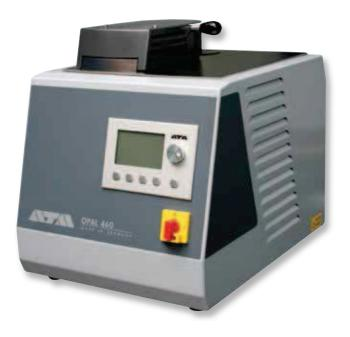
The **Opal 460** is a fully hydraulic, water cooled hot mounting press for mounting samples before polishing. The process sequence is executed automatically. The fully automatic sliding closure allows quick and easy opening/closing of the mould assembly. Mould assemblies can be exchanged quickly and without tools. The robust aluminium construction is powder coated. With its solid construction and ATM hydraulic system, the operating noise of the machine is minimized.
