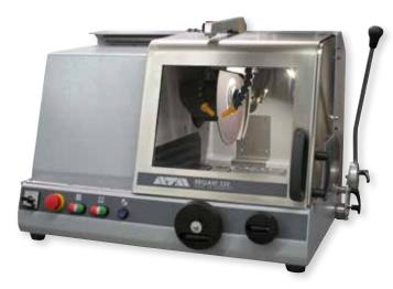
The **BRILLANT 230** is a wet abrasive cut-off machine with fine dynamic, manual wheel movement into samples up to  $\varnothing$  110 mm.
