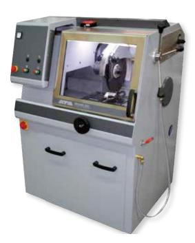
The universal wet abrasive cut off machine BRILLANT 255 with manual travel and fine dynamic cuting allows precise, soft touch cutting with 2 axes in arbitrary directions (Y/X axis) and can be equipped with a manual Z-axis for parallel serial cuts (option). Side openings allow cutting continuous long parts in the spacious cutting chamber of this solid and powder-coated aluminium construction.
