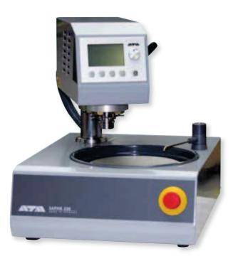
The **SAPHIR 520** is a single wheel grinder and polisher with top-mounted grinding and polishing head Rubin 500 for working wheels  $\emptyset$  200 - 250 mm.
