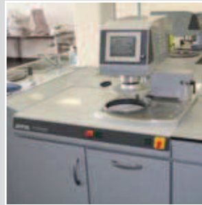
HIGH SPEED GRINDER SAPHIR 375
