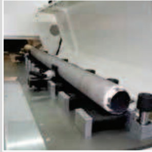
AUTOMATIC CUT-OFF OF SPUN IRON PIPES
