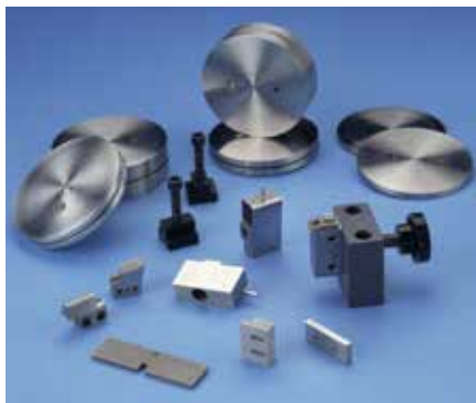
Fig. 7 Optional weight sets, clamps, anvils, and striking tups.
