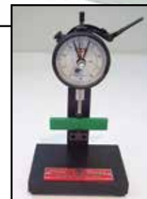
Fig. 9 Model 799 Notch Depth Verification Device.
